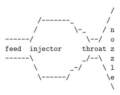
The converging portion at the throat is shallower (hence longer) than the diverging portion at the injector face.
